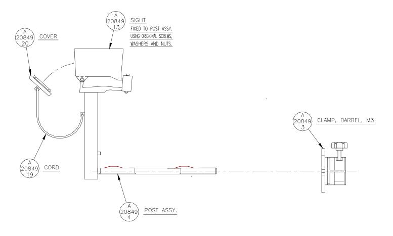
Fig 2 Parts list for DZD-M3M-01 & M2-01
